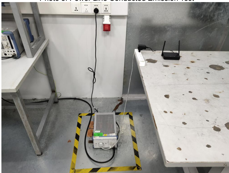
FCC ID: 2ADFS-LR01 Photo of Power Line Conducted Emission Test
