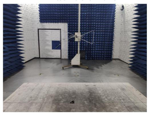
RADIATED EMISSION TEST SETUP ABOVE 1GHZ
