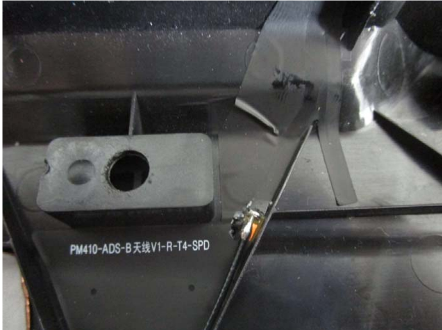
EUT- Right ADS-B Antenna Right View
