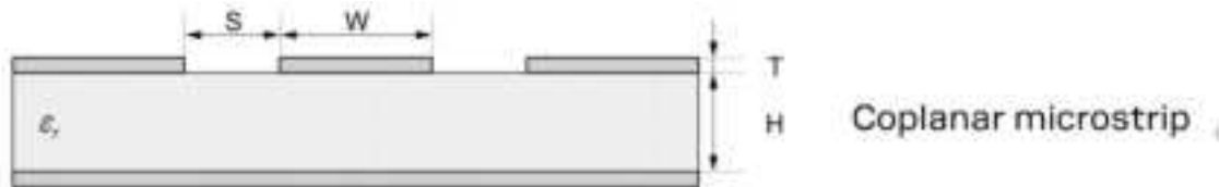
Figure 25: Coplanar micro-strip dimension specification
