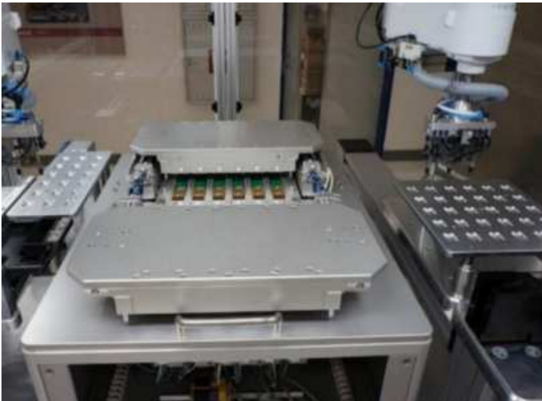
Figure 21: Automatic test equipment for module test
