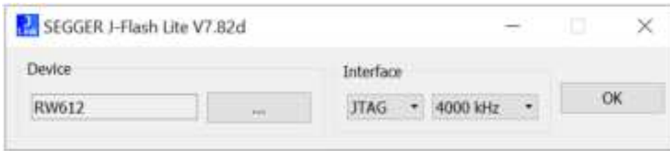
Figure 15: J-Flash Lite device over JTAG interface
