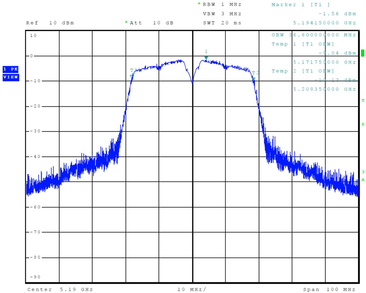
Figure 24 Plot of 99% Occupied Bandwidth 5150-5250 MHz Mode 12 U-NII-1 (802.11ac80)
