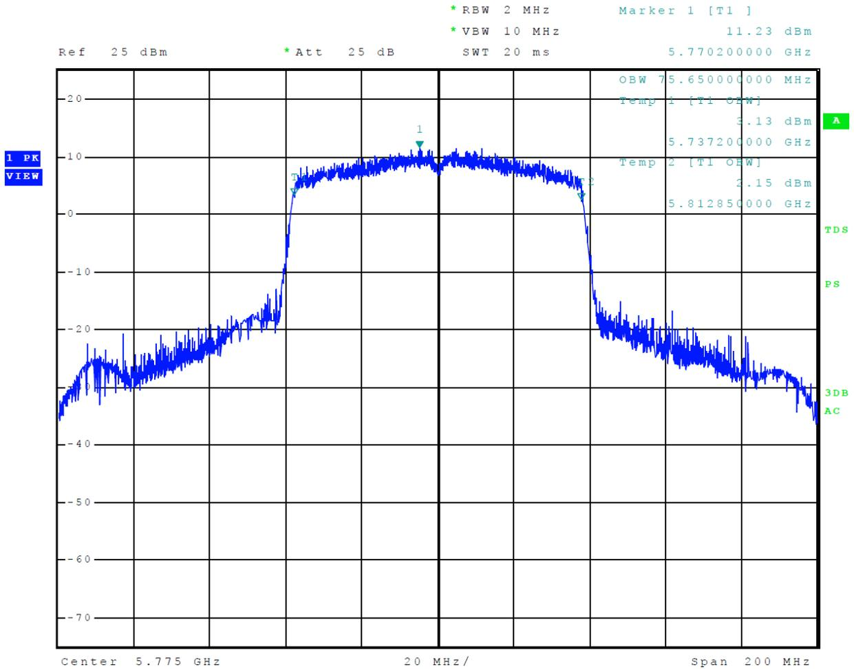
Figure 41 Plot of 6-dB Occupied Bandwidth 5725-5850 MHz Mode 13 U-NII-3 (802.11a)
