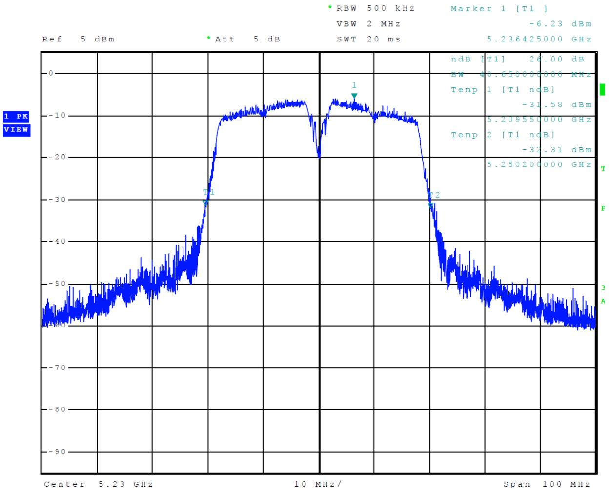
Figure 20 Plot of 26-dB Occupied Bandwidth 5150-5250 MHz Mode 12 U-NII-1 (802.11ac80)
