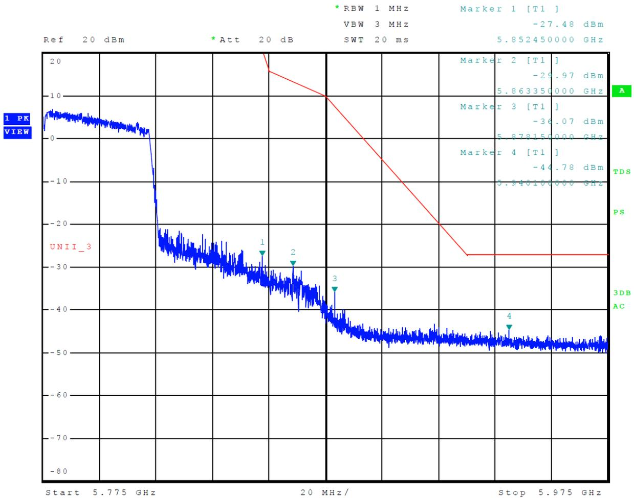
Figure 37 Plot of 99% Occupied Bandwidth 5725-5850 MHz Mode 13 U-NII-3 (802.11a)
