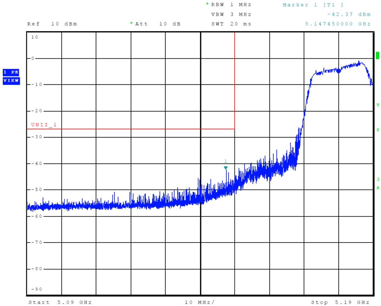
Figure 12 Plot of Lower Band Edge Across 5150-5250 MHz Mode 12 (802.11ac80)
