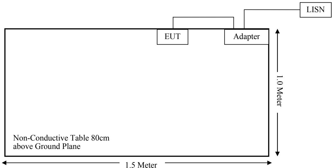
For Radiated Emissions(Below &amp; Above 30MHz):
