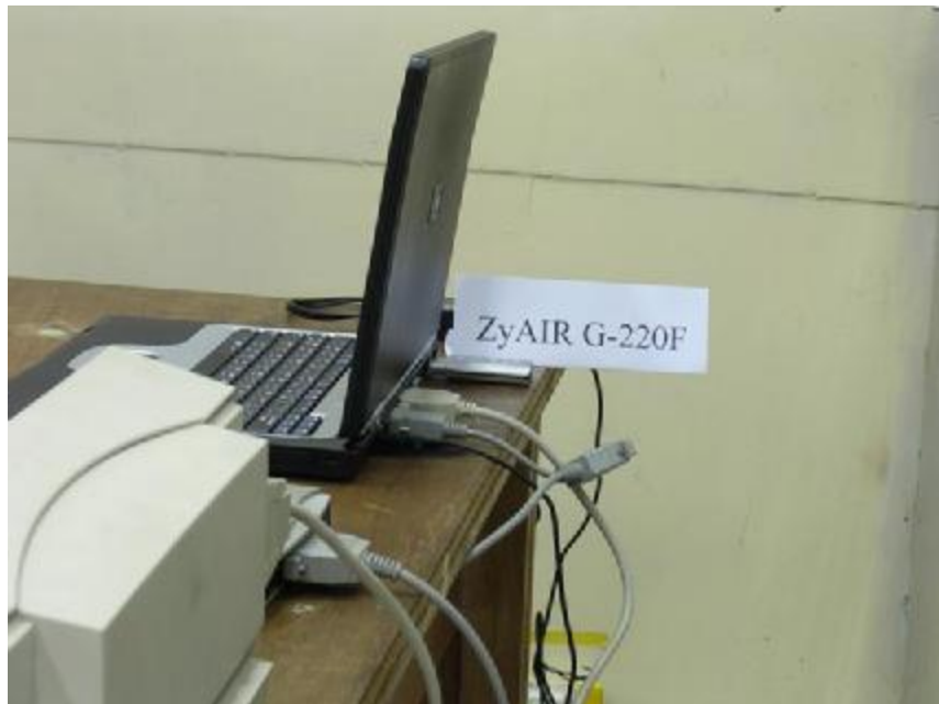
Photo 2: Conducted Emission Test Set-up photo
