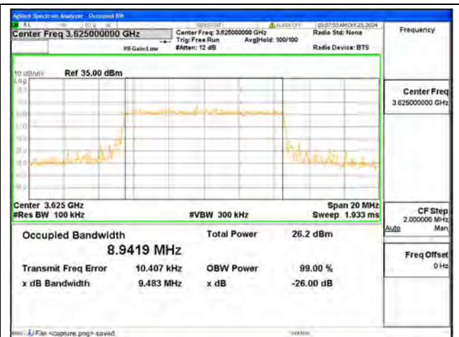
B48 / 10MHz / 16QAM/ Mid CH
