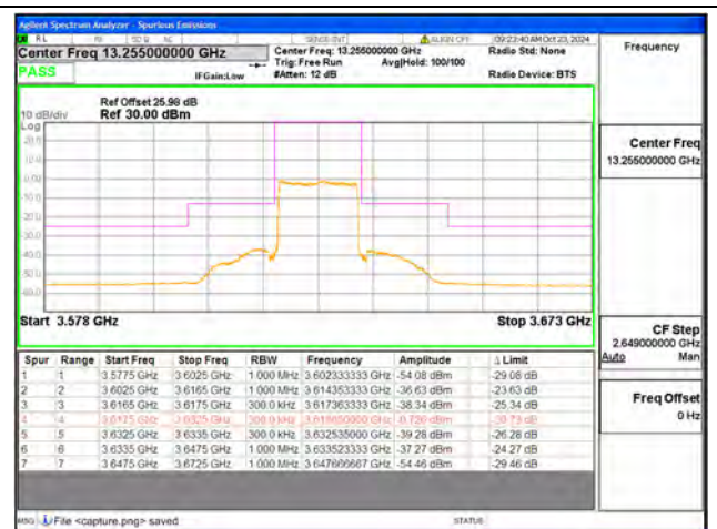
B48 / 15MHz / Mid CH / QPSK / FULL RB
