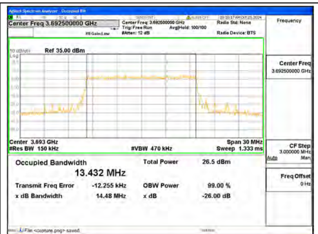
B48 / 15MHz / 16QAM/ High CH
