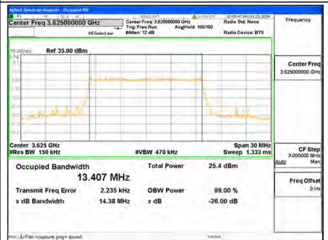
B48 / 15MHz / 64QAM/ Mid CH
