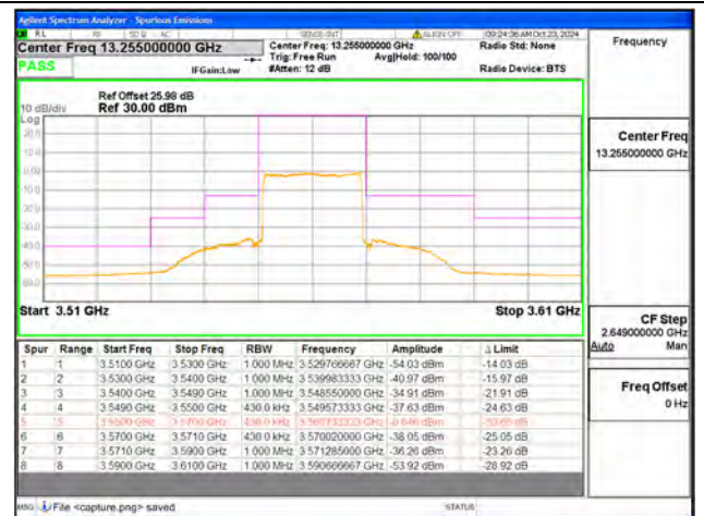
B48 / 20MHz / Low CH / QPSK / FULL RB
