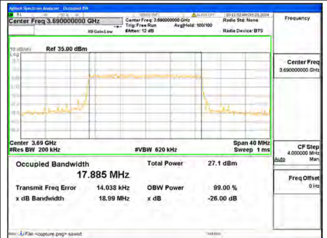
B48 / 20MHz / QPSK/ High CH
