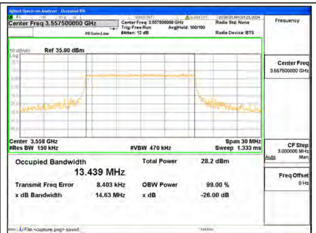
B48 / 15MHz / 16QAM/ Low CH
