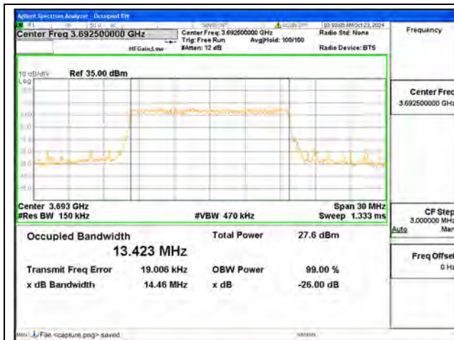
B48 / 15MHz / QPSK/ High CH
