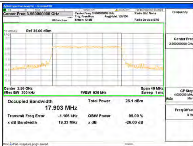
B48 / 20MHz / 16QAM/ Low CH
