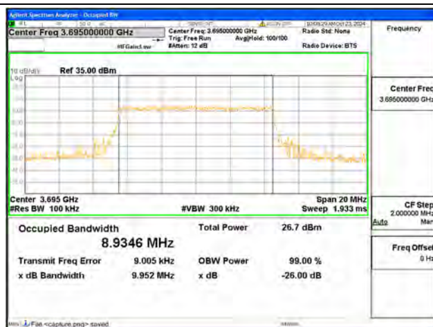
B48 / 10MHz / 16QAM/ High CH
