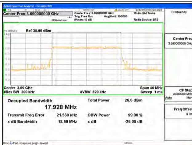
B48 / 20MHz / 16QAM/ High CH
