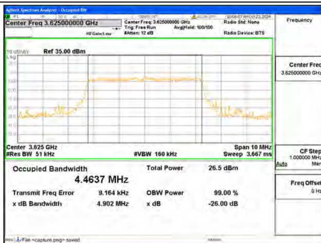
B48 / 5MHz / 16QAM/ Mid CH
