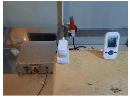
Radiated Emissions (30MHz-1GHz) Test Setup
