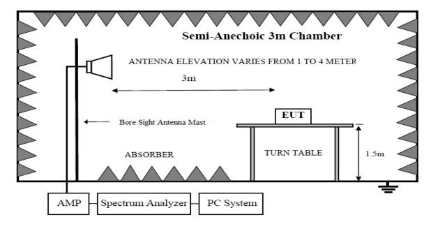
In Semi Anechoic Chamber (3m) Test Setup Diagram for Above 1GHz
