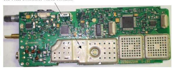
UHF P1225 Top Side showing heat spreader with thermal tape.
