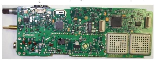
UHF P1225 Bottom Side with RF PA shield.
