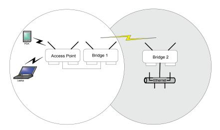
The following chart maps the basic procedure to be followed in configuring the three units as shown above. Essentially, you can follow the procedure as laid out in the section on point-to-point bridging. It is the BSSID and the Bridging Encryption that allows the two bridges to communicate. Needless to say, the configuration of the access point determines the functioning of the dependent WLAN.
