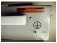
This closeup shows the ground and one of the seals that are standard on the FIPS 140-2 compliant 3e-531AP. Note that the ground will be installed permanently on installation of the unit and should not be disturbed after that.
