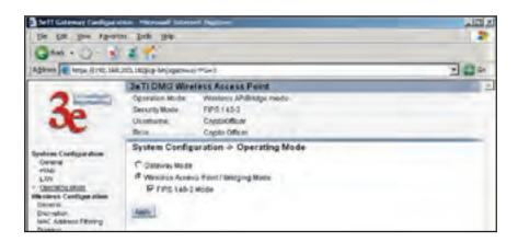
You can then proceed to change the management screens as necessary to reconfigure the device as a gateway. Configuration in gateway mode allows you to set firewall parameters. This is the main difference between the screens you will see in gateway mode and those covered in access point setup as discussed in Chapter 3.
