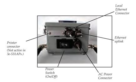
An AC Power Connector (not provided) can be plugged into an AC outlet. In some situations, the installation design may include elimination of the ability to plug the unit into an AC outlet. In such circumstances, the AC power is supplied (that is, hardwired) using the same AC Power Connector port. Usually, in the default configuration of the 3e-531AP, the AC Power Connector is not actively used. The socket outlet must be installed near the equipment and be easily accessible.
