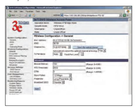
If you have the 3e AP configured in any mode *except* FIPS, setting TX Pwr Mode to **O**ff will only shut off the power on that one AP.
