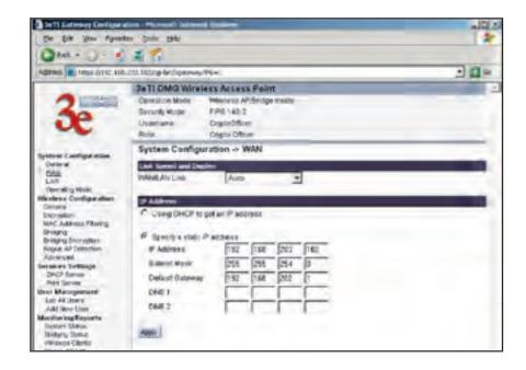
If not using DHCP to get an IP address, input the information that the access point requires in order to allow the wireless devices it controls access to the wired LAN. This will be the IP address, Subnet Mask, Default Gateway, and, where needed, DNS 1 and 2.
