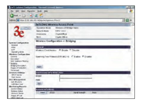
The Wireless Configuration — Bridging Encryption page is used to configure static encryption keys for the wireless bridge. This is an important page to set up to ensure that your bridge is working correctly. The encryption key that you use on this screen must be the same for any bridge connected to your bridging network in order for communication to occur. And on this screen, you can only select either a static 192 bit 3DES key or an AES key of either 128-bit, 192-bit, or 256-bit.
