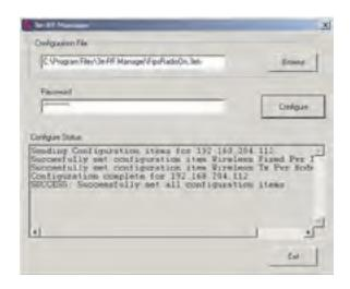
If any part of your update has failed, the Configure Status window will show you that it has failed in part or in whole and direct you to the area of the configuration file that you need to fix.
