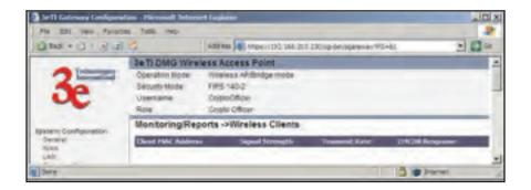
If Transmit power is disabled, either by setting TX Pwr Mode to Off on the management screen or by using the RF Manager (Chapter 7), the Wireless Clients page will show the results from each associated client in the EMCON Response column. If the client responds to the "disable" command, a **Yes** is displayed. If the column contains a **No**, this can mean either:
