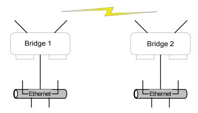
For the two bridges that are to be linked to communicate properly, they have to be set up with compatible commands in the setup screens.
