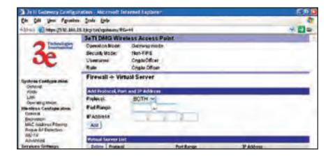
**Protocol** – Selection of either **UDP**, **TCP**, or **Both** (TCP and UDP) allows these specified network protocols to pass through during the TCP port communication with each virtual server IP address.
