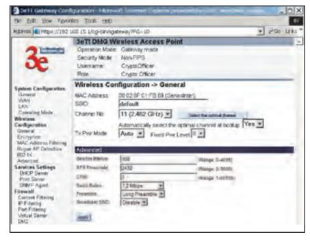
On the **Wireless Configuration** — **General** page, you must enter the SSID for the wireless LAN. This is also where you can assign a channel number to the AP (if necessary) and modify the Tx Pwr Mode. There are some advanced options which are detailed in the chart below.
