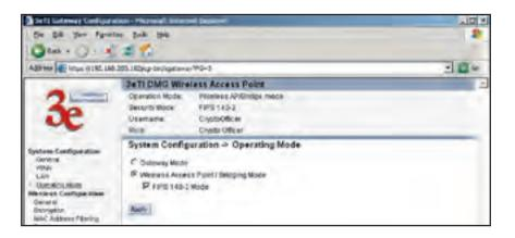
Select the radio button for **Wireless Access Point/Bridging Mode** and click **Apply**. If you wish to use Advanced Encryption, check the FIPS 140-2 Mode option. The unit will reboot. You do not need to log back on. After reboot, an instructional page will appear and you can then navigate back to the Management Module main screen.
