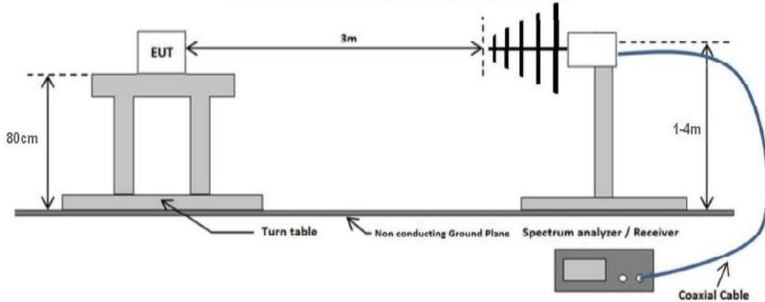
**Radiated emissions test setup above 1 GHz**
