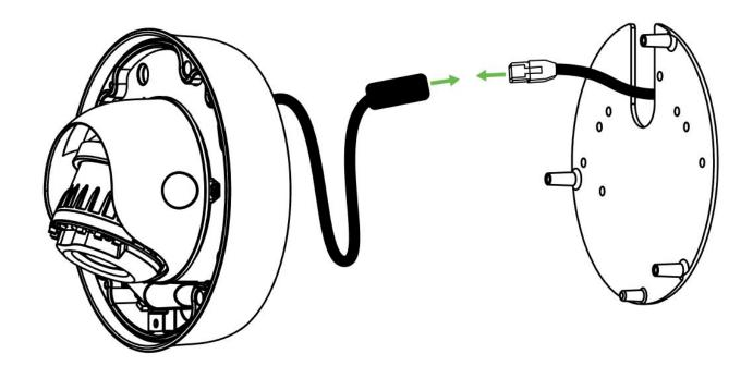
6. Mount camera to mount plate with 3x captive security torx screws using the provided tool.
