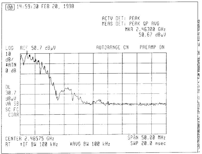
PAGE 12.2. EMISSIONS PINNACLE COMMUNICATION, INC., LUCENT DSW CARD 2.4GHZ NSU EIPRTR 1998-FEB-20, 14:03, FRI PARABOLIC ANTENNA
