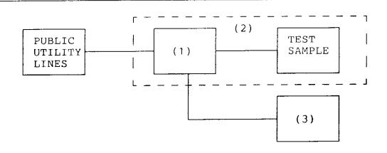
(1) LINE IMPEDANCE STABILIZATION NETWORK
