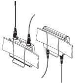
The transmitter is attached to clothing (e.g. belt, waistband) with the supplied belt clip. The clip is detachable so that you can also
