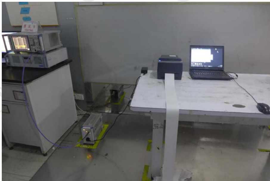
CONDUCTED EMISSION TEST SETUP
