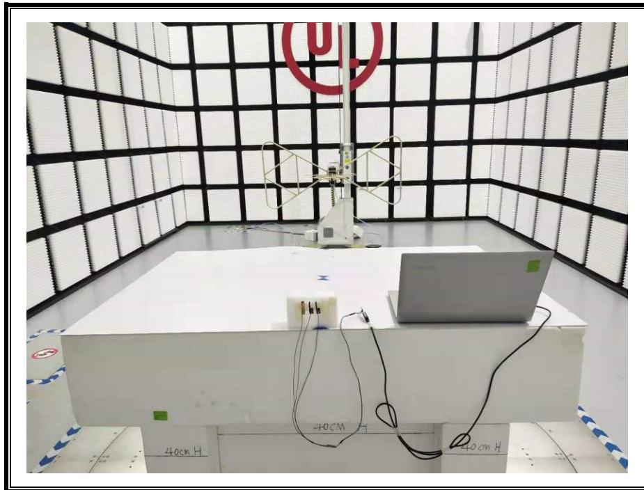
RADIATED RF MEASUREMENT SETUP (Below 30MHz)
