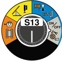
The selector S13 selects the operating mode of the machine. When changing the operating mode, press START to enable it. When activated, this switch must be in Positioning mode.
