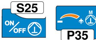
The Pump command is enabled with selector S25 (push-push command).
