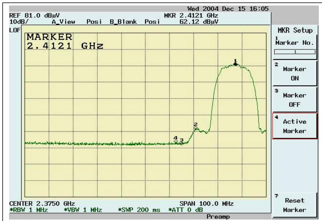
Band Edge measurement for radiated emission in Restricted Band(Radiated)
