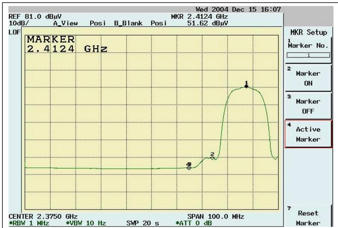
**Band Edge measurement for radiated emission in Restricted Band(Radiated) Peak Mode (Channel 11)**
