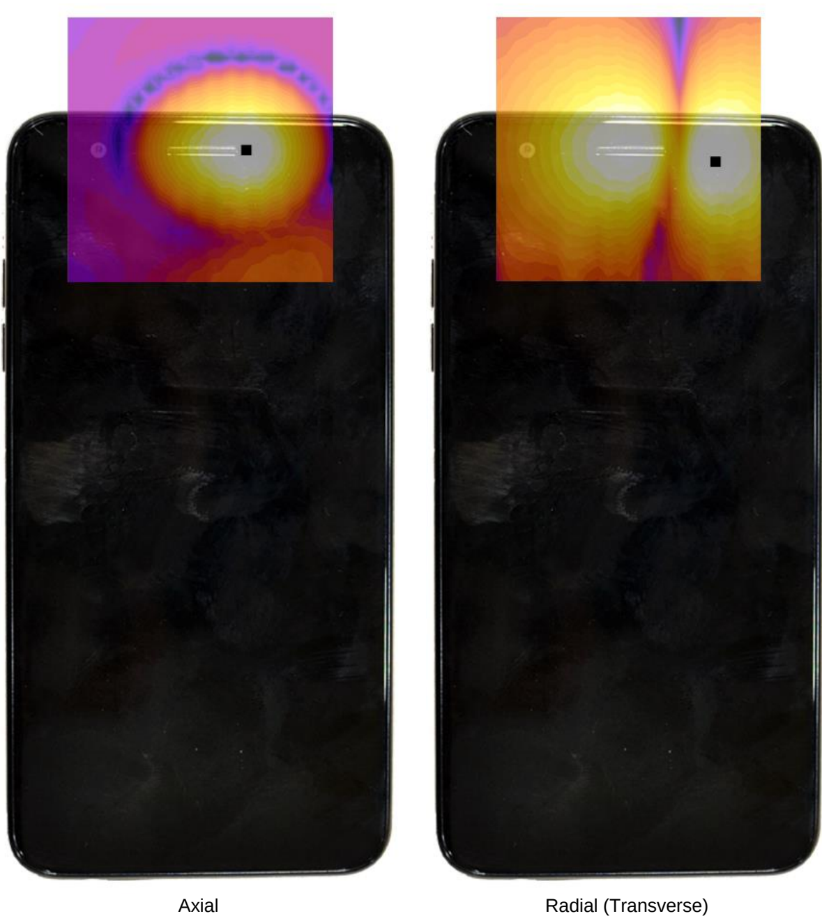
Figure 16-3 T-Coil Scan Overlay Magnetic Field Distributions
