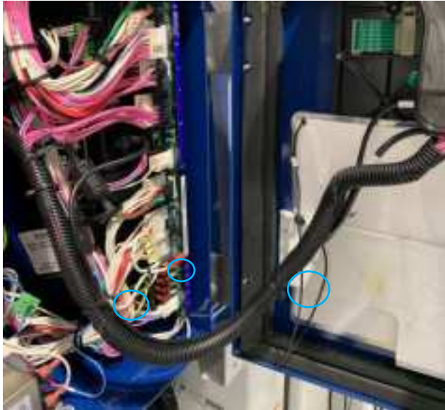
Figure 7a: Securing wire harness
