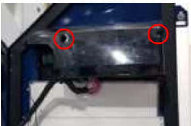
Figure 2a: Removal of Rain Shield
