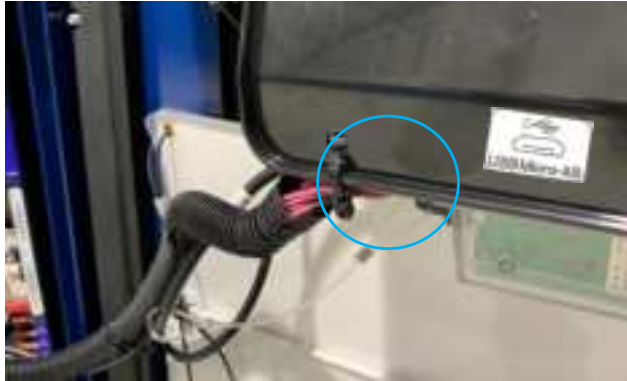
Figure 7c: Routing wire harness and label location
