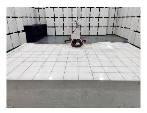
Set-up for Radiated Spurious Emission, Above 1GHz
