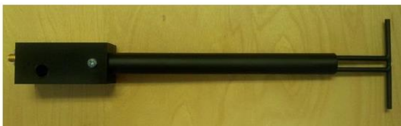
Figure 1 – MVG COMOSAR Validation Dipole
