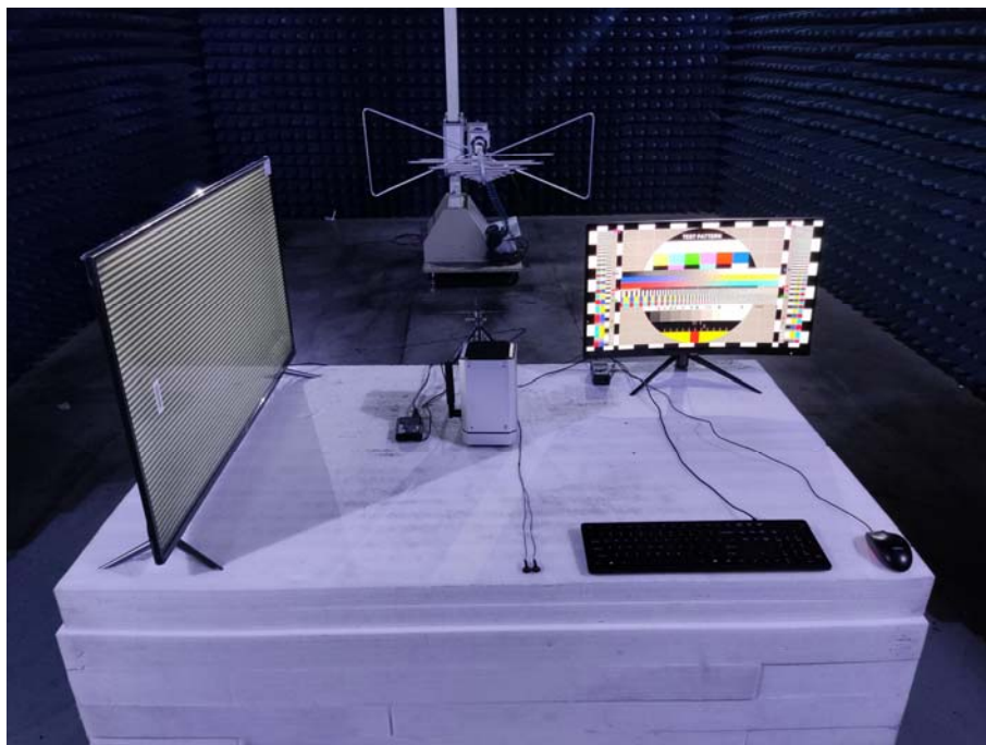
Photo of Radiated Emission Measurement (Below 1G) Adapter 1: HA-1600-12
