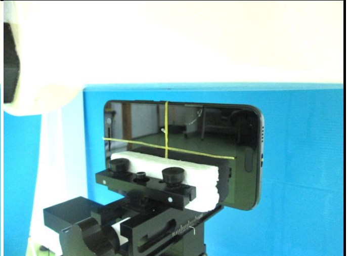
Right Side of EUT with 1.0 cm Gap
