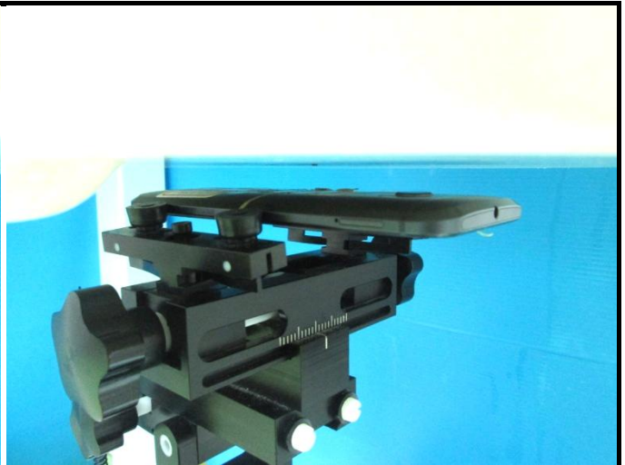
Rear Face of EUT with 1.0 cm Gap
