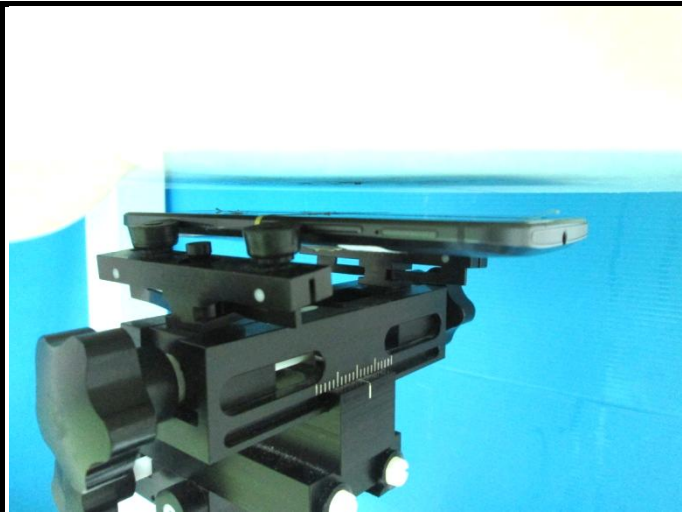
Front Face of EUT with 1.0 cm Gap
