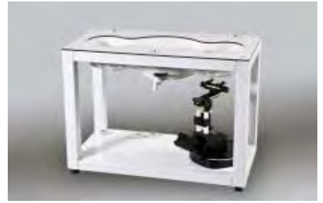
Figure E.5.1 SAM Twin Phantom
