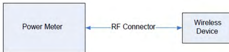
Figure 6.1.1 Power Measurement Setup
