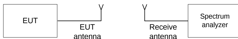
Figure 7.7.1 Band edge emission test setup
