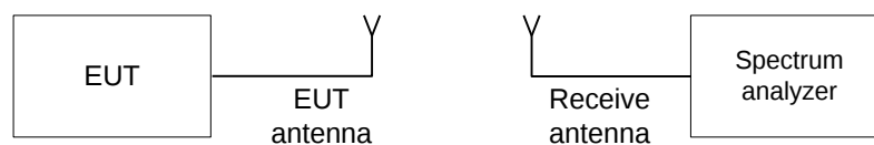
Figure 7.1.1 The 20 dB bandwidth test setup
