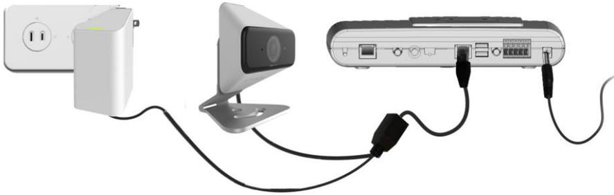
**Figure 1: Camera Installation**
