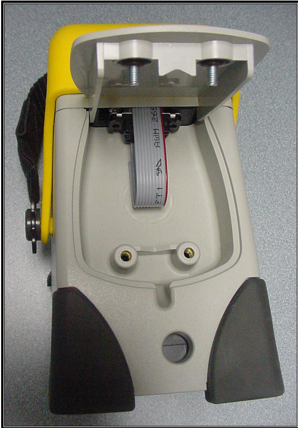
PHOTOGRAPH 11: EUT BACK COVER OPEN SHOWING DATA CABLE
