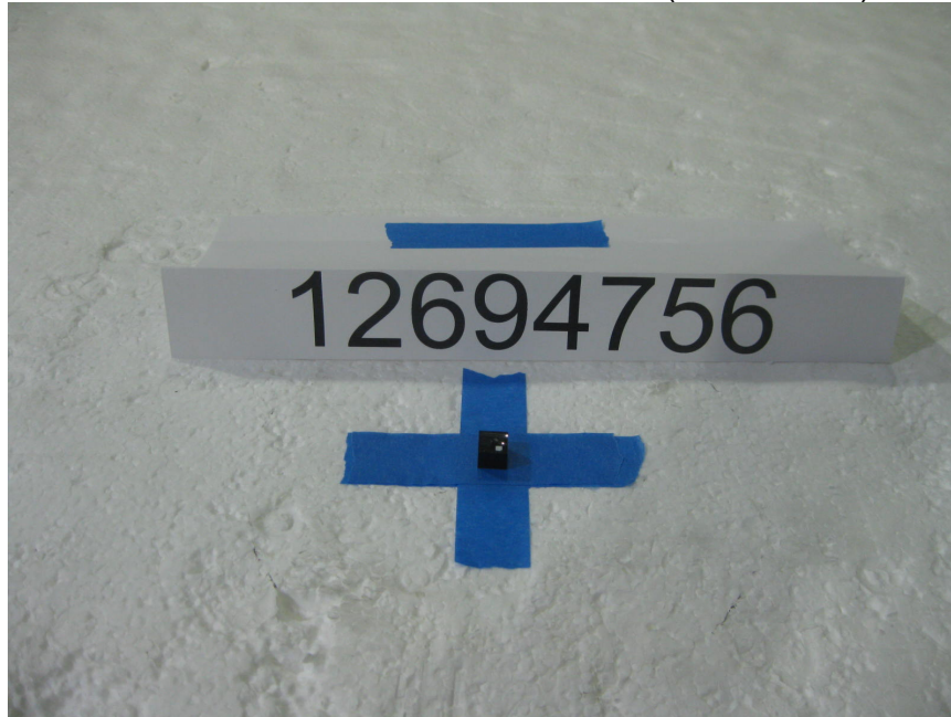
RADIATED SPURIOUS EMISSIONS SETUP (Above 1GHz)
