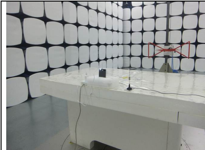
Radiated Spurious Emissions Test Setup Below 1GHz
