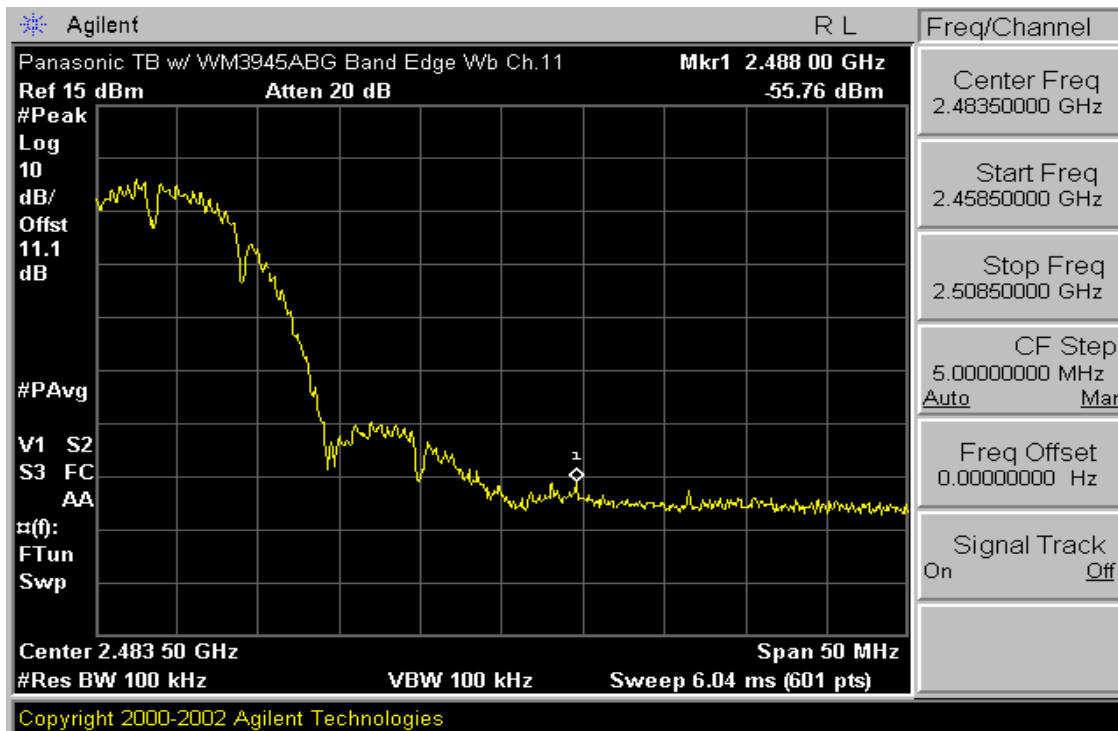
Plot 6-20. Band Edge Plot (802.11b – Ch. 11)
