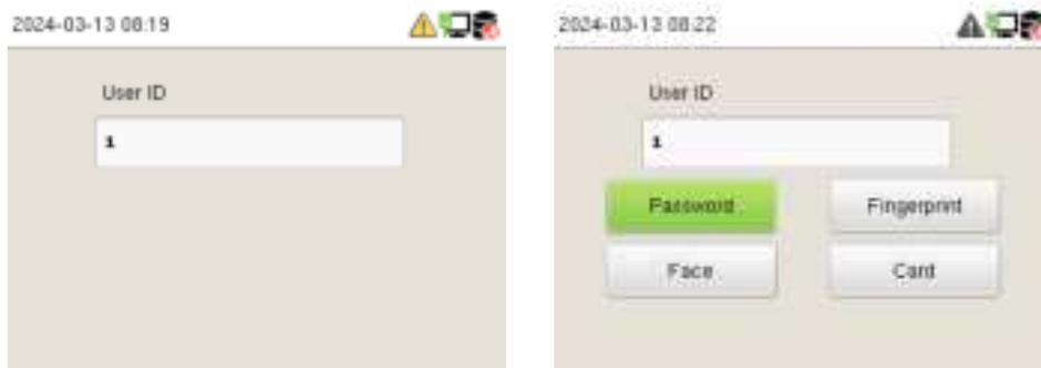
If an employee registers a fingerprint, face and card in addition to the password, the following screen will appear. Select **Password** to enter card verification mode.
