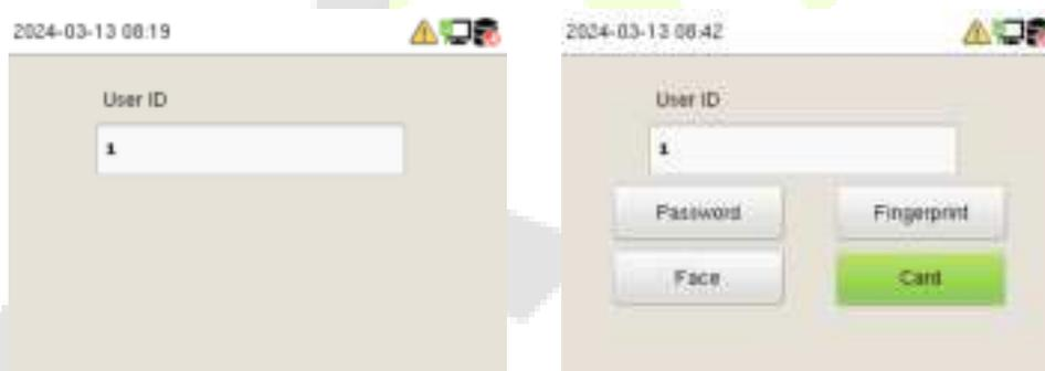
If an employee registers a fingerprint, face and password in addition to the card, the following screen will appear. Select **Card** to enter card verification mode.
