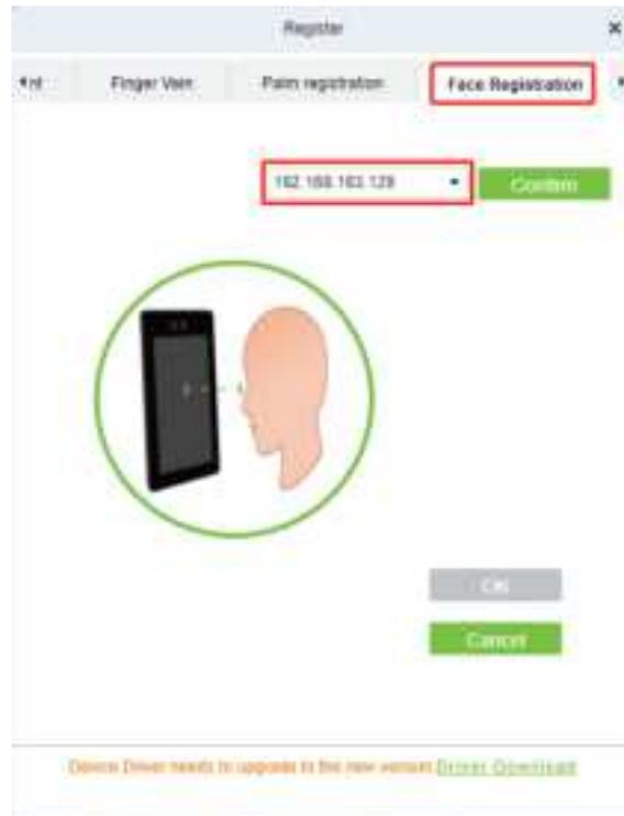
9. After the device prompts "Face registration begin", face towards the camera and keep the face in the centre of the screen and stay still during face registration. If the face is successfully registered, the device will prompt "Registered successfully".
