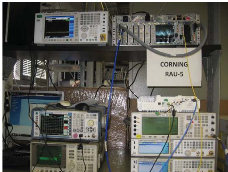
Figure 3. Conducted Emission From Antenna Port Tests
