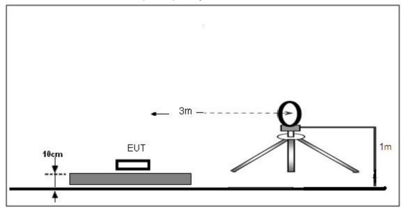
(B) Radiated Emission Test-Up Frequency 30MHz~1GHz
