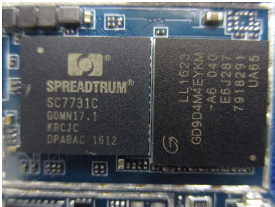
EUT- Main Chip View
