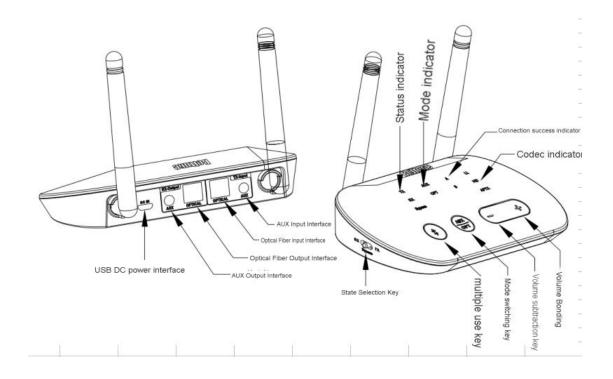
USB DC Power Supply Port / AUX Output Port / SPDIF Output Port / SPDIF Iinput Port / AUX Input Port
