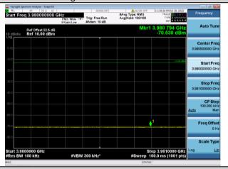
5G NR (3700-3800MHz) \_ SCS 30K Intra-band Continuous CA, Nominal Bandwidth: 10M+10M+10M+10M+10M+10M \_ Low channel+ High channel
