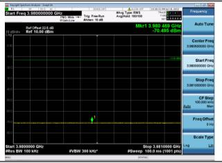
5G NR (3700-3800MHz) \_ SCS 30K Intra-band Continuous CA, Nominal Bandwidth: 40M+40M \_ Low channel+ High channel
