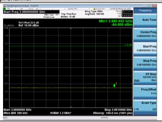
5G NR (3700-3800MHz) \_ SCS 30K Intra-band Continuous CA, Nominal Bandwidth: 20M+20M+20M \_ Low channel+ High channel
