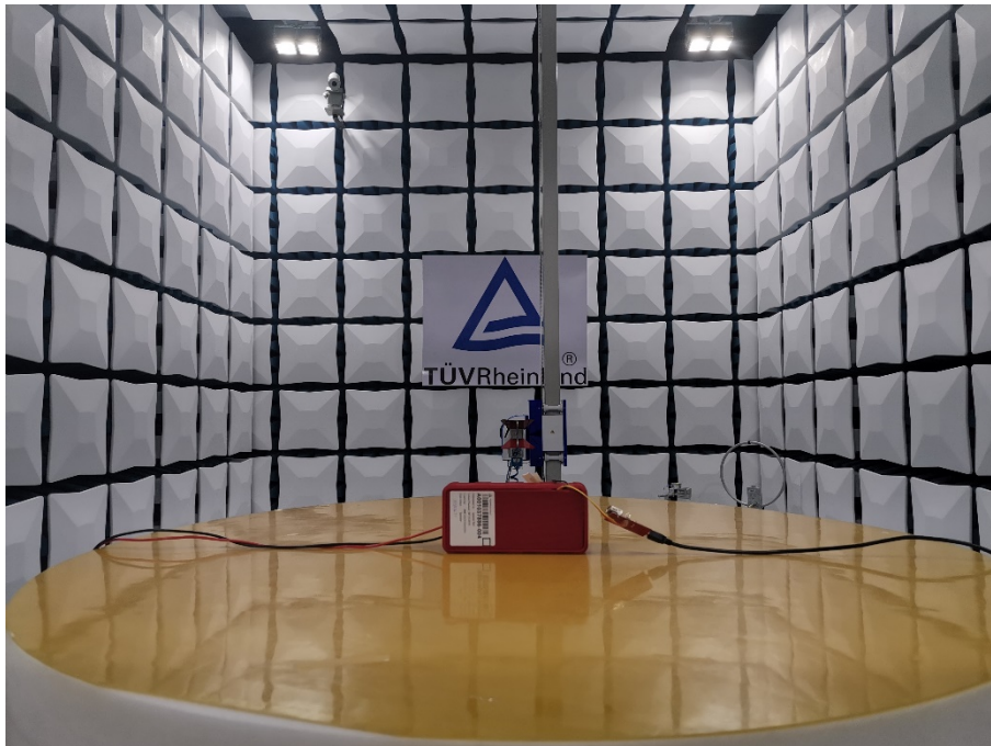
Photograph 2: Set-up for Radiated Spurious Emission, Above 1GHz
