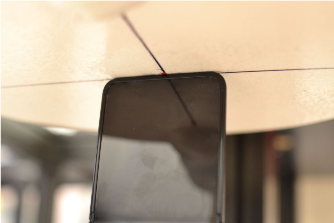
SAR Test Setup Photo 16 – Phablet, Bottom Edge, 0 mm
