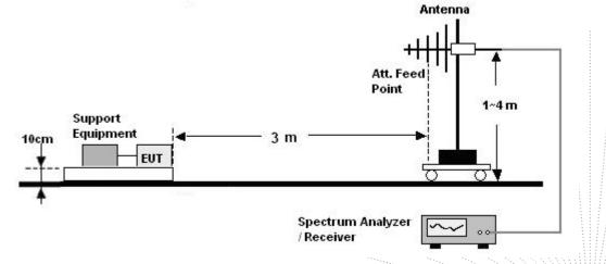
(C) Radiated Emission Test-Up Frequency Above 1GHz
