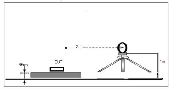
(B) Radiated Emission Test-Up Frequency 30MHz~1GHz
