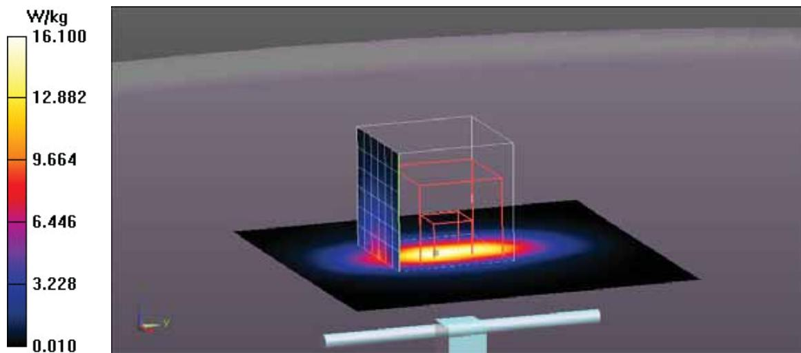
**Test Laboratory: Eurofins Product Service GmbH****System Performance Check - ELI Phantom - EX3DV6 - MSL - 2450 MHz 24-01-2017****DUT: Dipole 2450 MHz; Type: D2450V2; Serial: 722**
