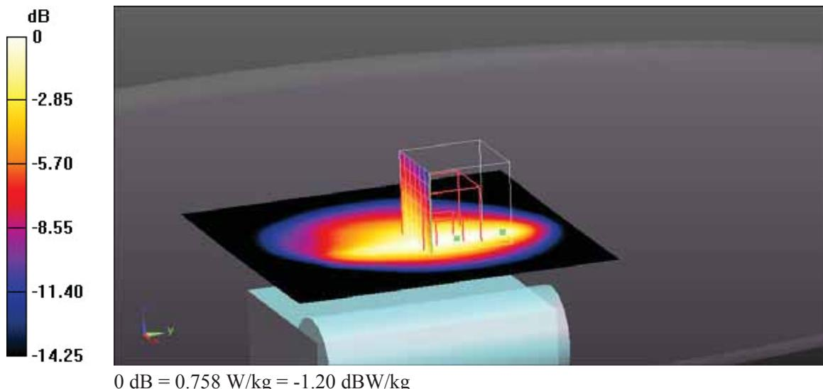
**Test Laboratory: Eurofins Product Service GmbH****GSM 1900 - Ch. 661 - 2xSlot - BOTTOM 0mm****DUT: Asthma Monitor AM3; Type: AM3 Option G+; Serial: -**Communication System: UID 0 - n/a, GPRS 1900 2xSlot; Frequency: 1880 MHz; Duty Cycle: 1:4.14954
