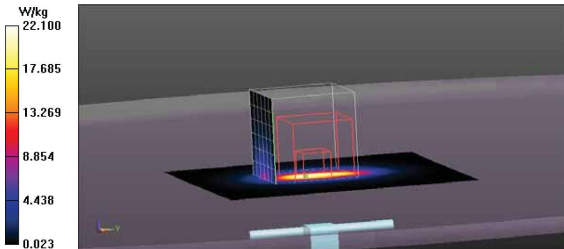
**Test Laboratory: Eurofins Product Service GmbH****System Performance Check - SAM Phantom - EX3DV4 - HSL - 900 MHz 10-01-2017****DUT: Dipole 900 MHz; Type: D900V2; Serial: 164**
