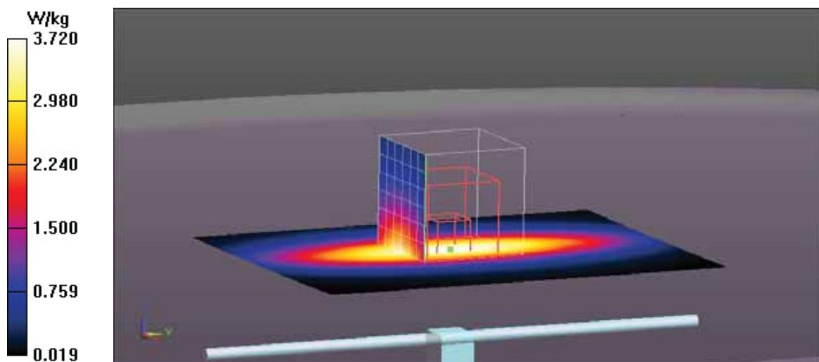
**Test Laboratory: Eurofins Product Service GmbH****System Performance Check - ELI Phantom - EX3DV4 - MSL - 900 MHz 17-01-2017****DUT: Dipole 900 MHz; Type: D900V2; Serial: 164**
