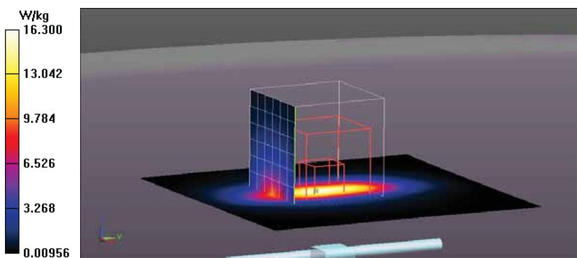
**Test Laboratory: Eurofins Product Service GmbH****System Performance Check - ELI Phantom - EX3DV6 - MSL - 1900 MHz 19-01-2017****DUT: Dipole 1900 MHz; Type: D1900V2; Serial: 5d025**
