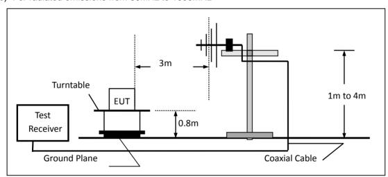
(c) For radiated emissions above 1000MHz
