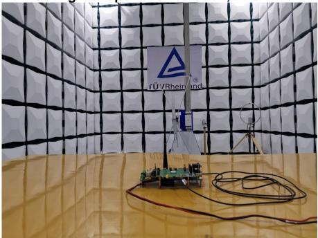
Set-up for Field Strength of Spurious Radiation, above 1 GHz
