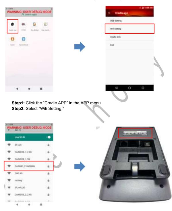
**Step3:** Find the SSID of the wifi signal brocasting by the POS cradle. The naming rule of SSID is "CASWIFI\_XXXXXXXX" The last 9 digits match the last 9 digits of the POS cradle serial number. The serial number could be found on the product label.
