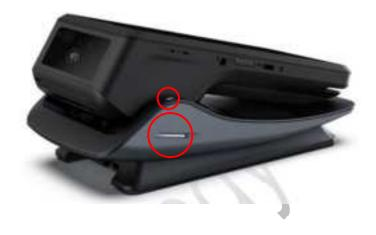
**Step1:** Plug the DC jack cable into DC jack connector on the rear part of S1F4B. **Step2:** The power indicator on the left fron side of S1F4B will light up immediately after plugging the DC jack.
