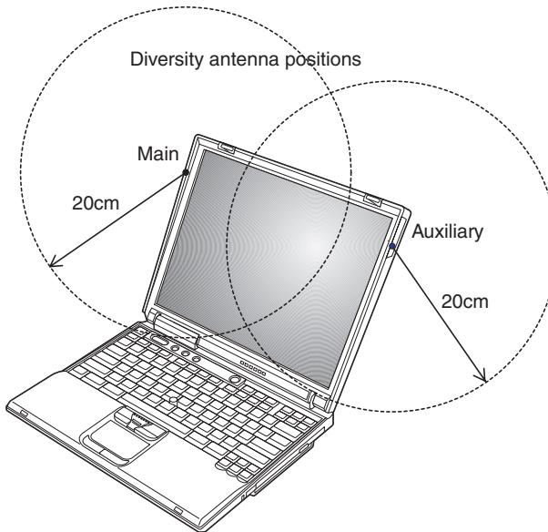
**Note:** The transmission diversity function is implemented for the Card. The function does not emit radio frequencies simultaneously from both antennas. One of the antennas is selected automatically or manually (by users) to have good quality of radiocommunication.
