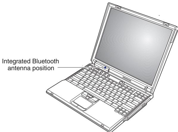
The antenna of IBM Integrated Bluetooth with 56K Modem is located in the left hinge portion of keyboard. Transmitted energy from the Bluetooth device is very low compared to other RF devices. Therefore a 20 cm separation from the Bluetooth antenna is not required.
