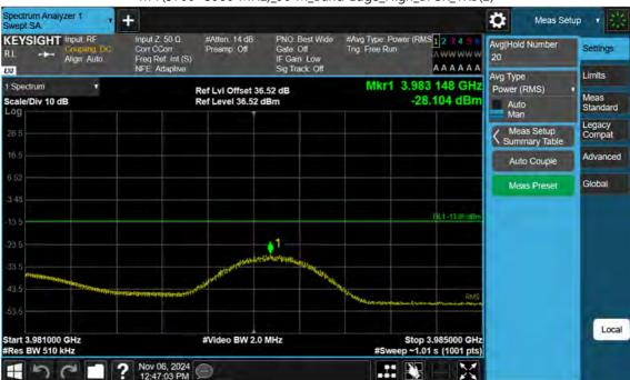
n77(3700~3980 MHz)\_90 M\_Band Edge\_High\_BPSK\_1RB(2)
