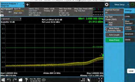
n77(3700~3980 MHz)\_90 M\_Band Edge\_Low\_BPSK\_1RB(2)
