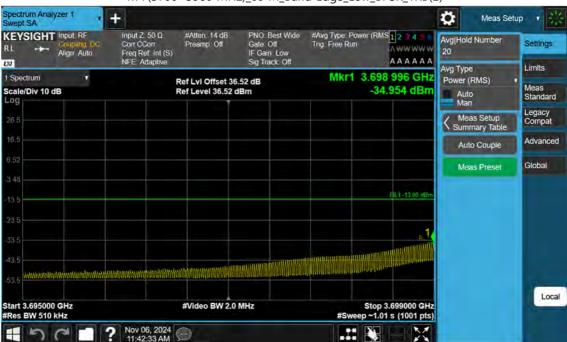
n77(3700~3980 MHz)\_60 M\_Band Edge\_Low\_BPSK\_1RB(2)
