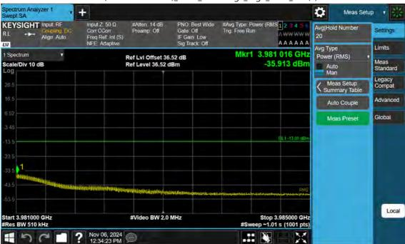
n77(3700~3980 MHz)\_80 M\_Band Edge\_High\_BPSK\_1RB(2)
