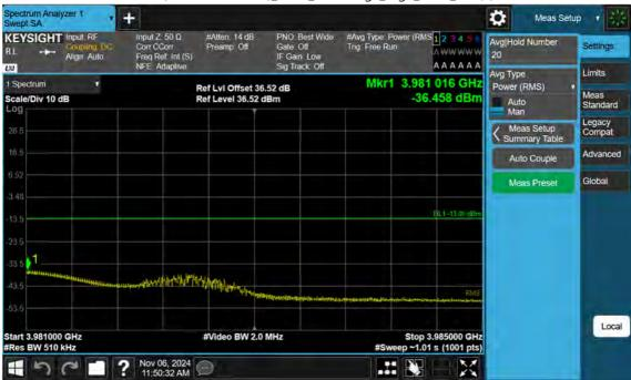
n77(3700~3980 MHz)\_60 M\_Band Edge\_High\_BPSK\_1RB(2)
