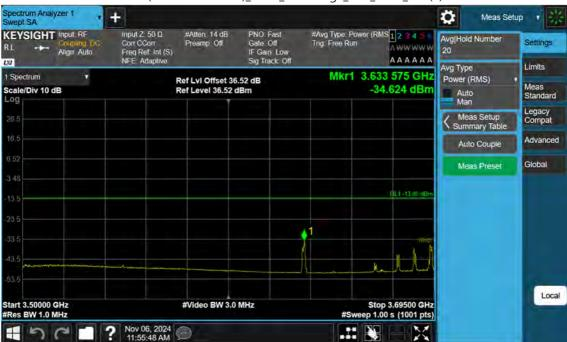
n77(3700~3980 MHz)\_70 M\_Band Edge\_Low\_BPSK\_1RB(3)
