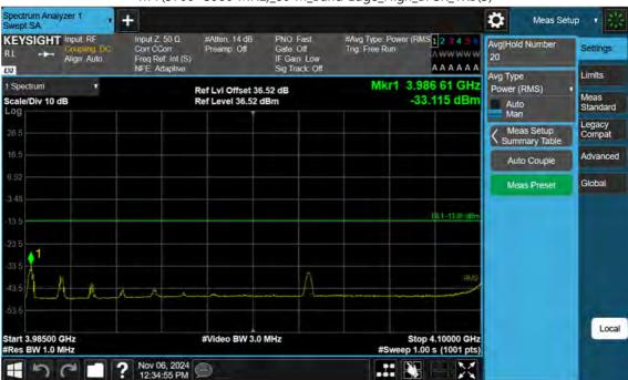
n77(3700~3980 MHz)\_80 M\_Band Edge\_High\_BPSK\_1RB(3)
