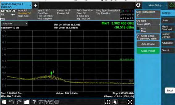
n77(3700~3980 MHz)\_70 M\_Band Edge\_High\_BPSK\_1RB(2)
