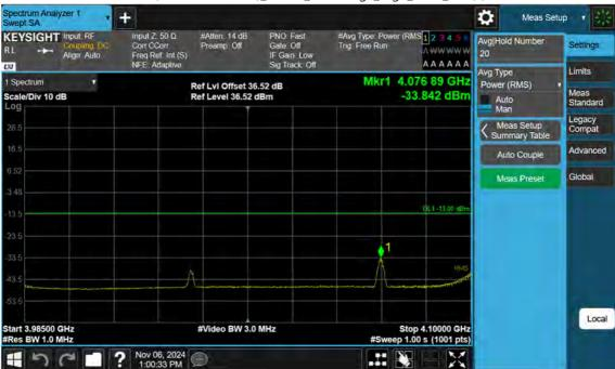
n77(3700~3980 MHz)\_100 M\_Band Edge\_High\_BPSK\_1RB(3)
