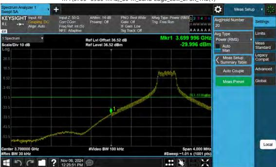
n77(3700~3980 MHz)\_80 M\_Band Edge\_Low\_BPSK\_1RB(1)
