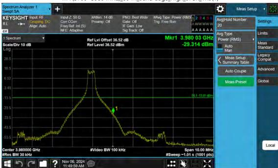
n77(3700~3980 MHz)\_60 M\_Band Edge\_High\_BPSK\_1RB(1)
