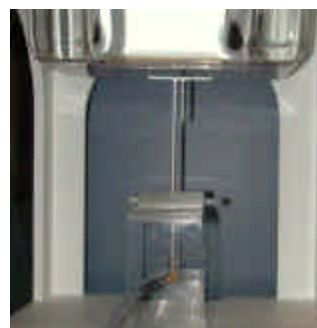
Figure A.0 Dipole Validation Test Setup
