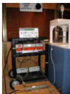
Figure A.0 Dipole Validation Test Setup
