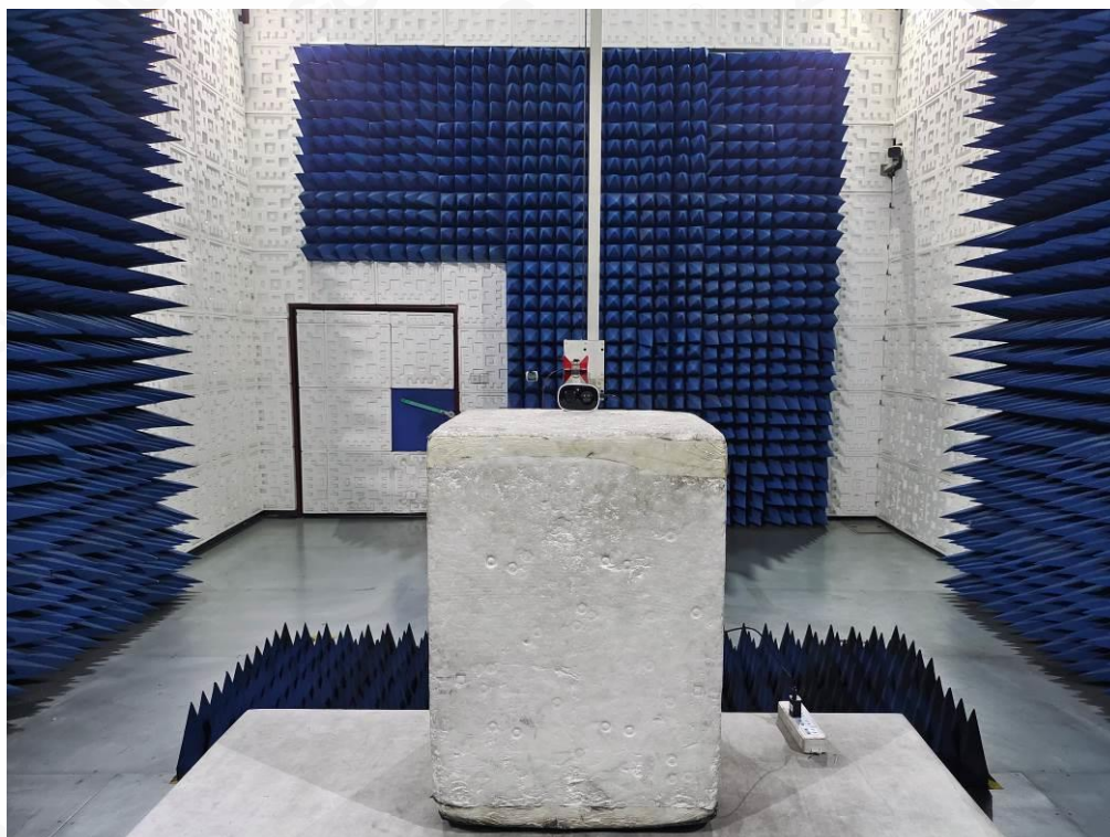
FCC RADIATED EMISSION TEST SETUP ABOVE 1GHZ
