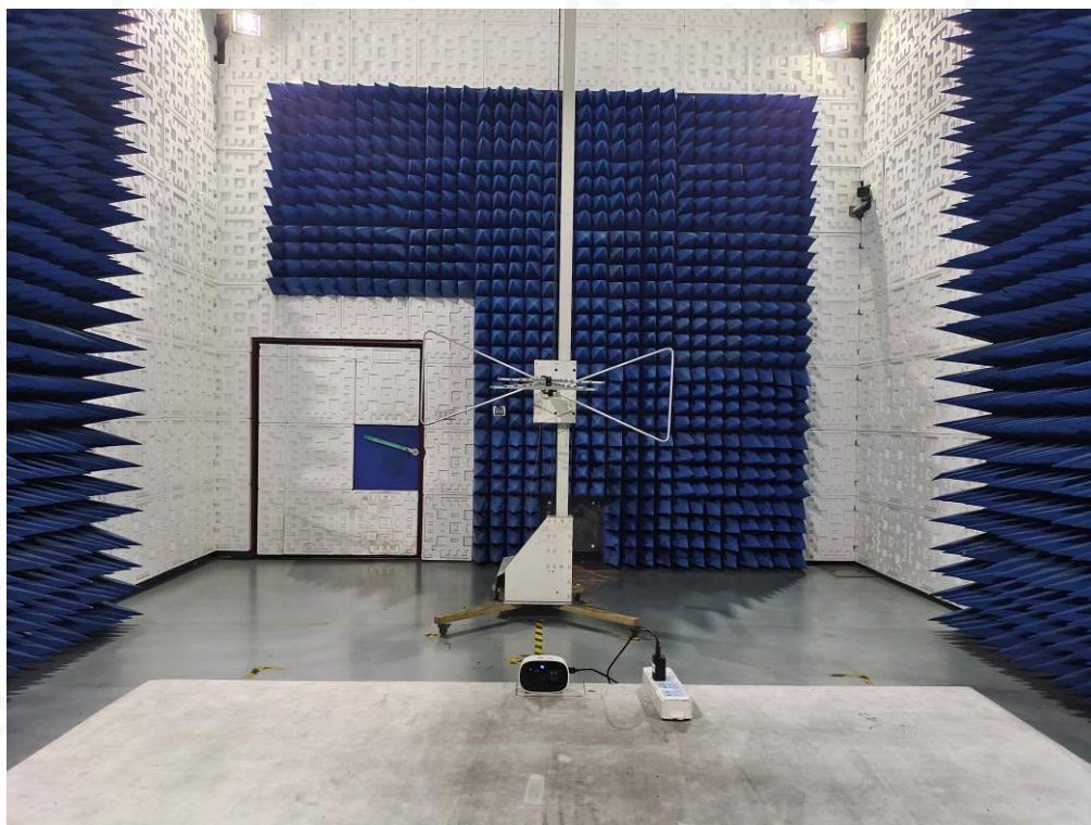
FCC RADIATED EMISSION TEST SETUP ABOVE 1GHZ
